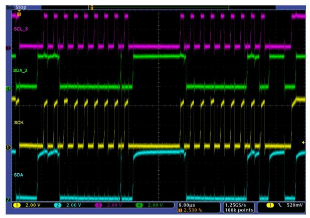
Figure 5. I<sup>2</sup>C Level Shifter Measurement
