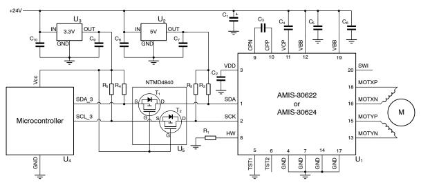
Figure 3. Application Example with Discrete Level Shifter
