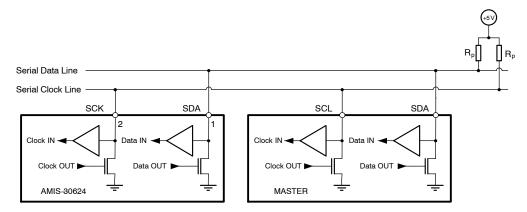
Figure 2. Connection to the I<sup>2</sup>C Bus
