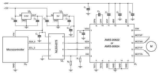
Figure 4. Application Example with 2-bit Level Translator
