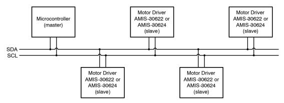
Figure 1. Example of an I<sup>2</sup>C Bus Configuration Using Four Stepper Motor Drivers (Note 1)
